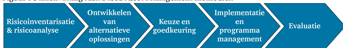
Figuur 1 Samenvatting Risk Based Asset Management methodiek
